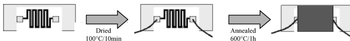
Fig. 7. Schematic representation of the screen-printing process.
